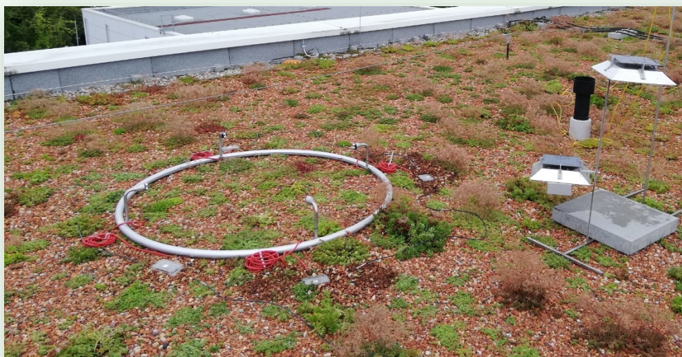
Fig .: Ultrasonic sensors and air temperature measurement (below) Author: N. Wollschläger (SUSOZ)
